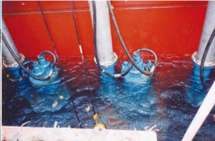
**GSZ-4:** High head, high volume drainage pump with internal 4-pole motor
