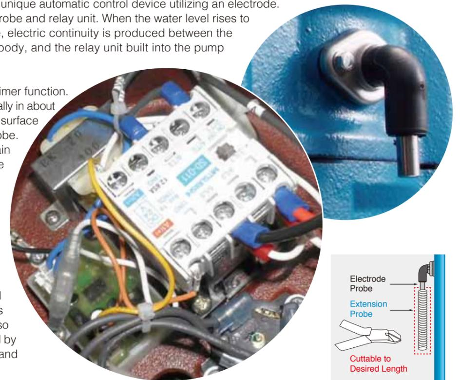
It is possible to set a lower starting water level by using an extension probe (optional accessory). The starting water level is adjustable because the extension probe can be cut to the desired length as it is made of coil spring.
