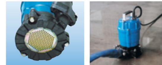
**LSC** Can drain water to 1mm in depth. A valve seat and swing check valve prevent suctioned water from backflowing.
