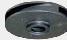
The closed impeller is adopted in the PSF-series. The impeller is also referred to as shrouded impeller, as it has circular shrouds at both sides of the impeller vanes. Although the pump has a limited solids passage capability, it can be used for higher pumping head applications.
